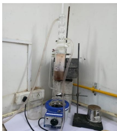
Figure 2: Soxhlet extraction of Blueberry
