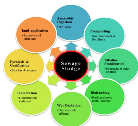
Figure 1: Overview of novel biological and biotechnological treatment strategies for SS, including anaerobic digestion, composting, bioremediation, and pyrolysis, with potential resource recovery outcomes.
